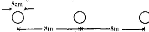
Calculate the inductance per phase per km. Compare for equal conductor area, the inductance of this system with that of bundle conductor system shown below
