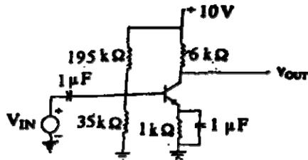
For the circuit shown above taking  $\beta = 200$  and  $V_{BE} = 0.6$  V
