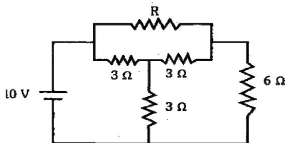
Determine the value of  $H$  shown in the above figure such that the  $6\ \Omega$ -resistor consumes the maximum power.
