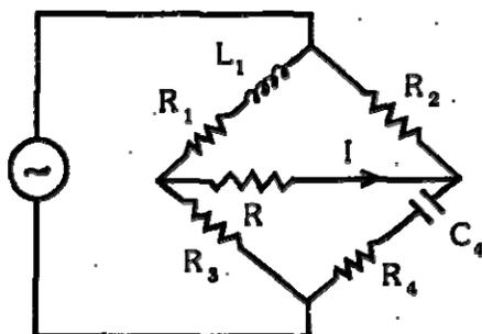
In the circuit shown above when  $I = 0$ , show that  $\omega L_1/R_1 = 1/\omega C_4 R_4$ .
