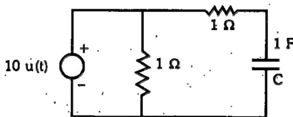
In the circuit shown above, determine the initial and final values of the current through the  $1\ \text{F}$ -capacitor. Make use of theorems.
