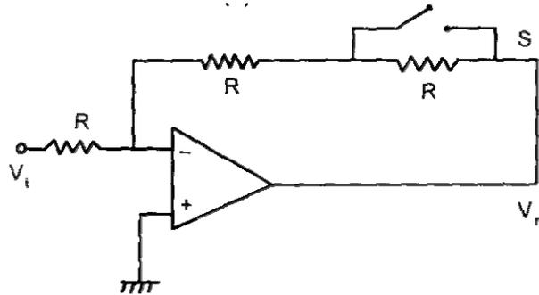
The magnitude of the gain in the inverting operational amplifier circuit shown above is Y, with the switch open. When the switch is closed the magnitude of the gain is
