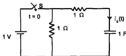
2. (a) In the circuit shown in the figure,  $S$  is closed at  $t = 0$ . Find the current  $i(t)$  through the capacitor at  $t = 0$ .
