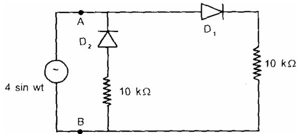
A voltage source  $V_{AB} = 4 \sin wt$ , is applied across the terminals A and B of the circuit above. The diodes are assumed to be ideal. The impedance offered by the circuit across the terminals A and B in kilo ohms is:
