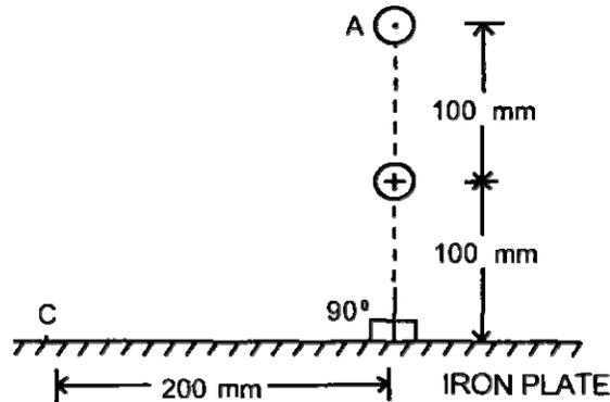
Calculate the magnetic field strength at a point C, 200 mm away from the bottom point on iron plate below the conductors. Also calculate the mechanical force per unit length on the conductor A.
