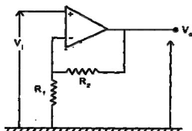
8. (a) Explain the operation of a Schmitt trigger circuit using an operational amplifier. Discuss the effect of hysteresis in such a circuit. 8
