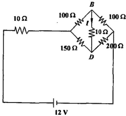
Calculate the current  $I$  flowing through the  $10\ \Omega$  resistor in the circuit shown above. Apply Thevenin's theorem.
