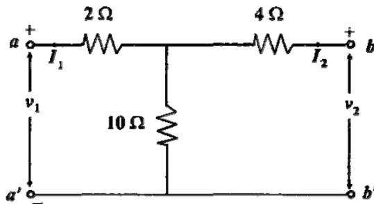
Find the ABCD parameters for the circuit shown above.
