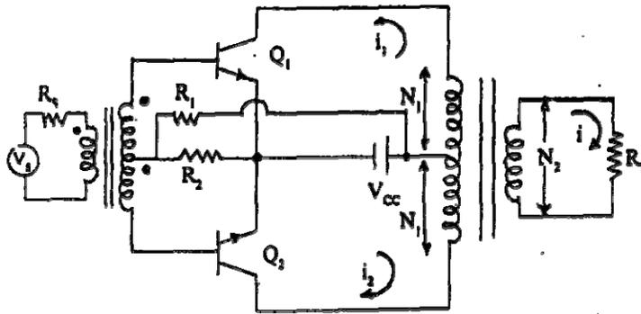
Give that  $R_2 = 0$ ,  $V_{CC} = 20\text{ V}$ ,  $N_2 = 2 N_1$ ,  $R_L = 20\ \Omega$  and the transistors have  $h_{FE} = 20$ . The input is a sinusoid. For the maximum output signal at  $V_m = V_{CC}$ , determine:
