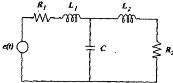
Obtain the state diagram for the network shown in the above figure. Write the state variable equation.
