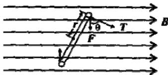
Write the Lorentz Force equation and explain its significance. Calculate the maximum torque of a rotor shown in the above figure when  $I = 60$  A,  $r = 8$  cm,  $B = 0.1$  web/ $\text{m}^2$  and length  $L = 12$  cm.
