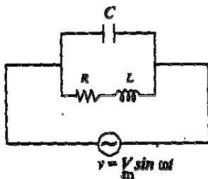
Find out the resonant frequency of the circuit shown above in terms of circuit parameters.
