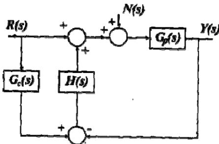
In a feedback control system shown in the above figure  $G_p(s)$  denotes the controlled process and  $G_c(s)$  and  $H(s)$  are the controller Transfer functions. There are two inputs namely  $R(s)$  and  $N(s)$
