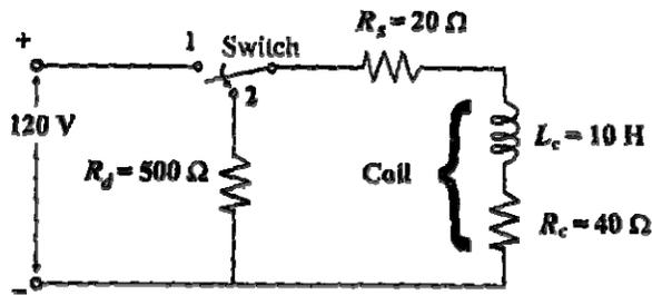
In the circuit shown above the switch is initially in position I. Find the voltage across the coil at the instant at which the switch is changed to position 2.
