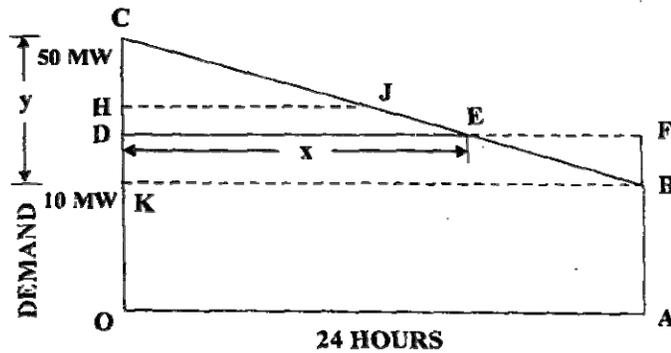
Fig 4 (b) : Load duration curve
