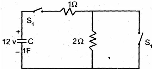
The capacitor in the circuit as shown above is initially charged to 12 V with  $S_1$  and  $S_2$  open.  $S_1$  is closed at  $t = 0$  while  $S_2$  is closed at  $t = 3$ . The waveform of the capacitor is represented by
