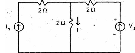
For the circuit shown above, the value of  $V_s$  is  $0$  when  $I = 4$  A. The value of  $I$  when  $V = 16$  V, is
