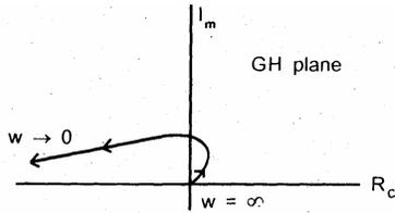
The Nyquist plot of a control system is shown above. For this system,  $G(s)H(s)$  is equal to
