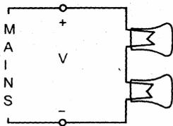
The incandescent bulbs rated respectively as  $P_1$  and  $P_2$  operation at a specified mains voltage are connected in series across the mains as shown in the above figure. Then the total power supplied by the mains to the two bulbs is
