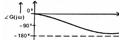
The Bode phase angle plot of a system is shown above.
