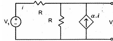
Consider the circuit as shown above which has a current-dependent current source. The value  $V_2/V_1$  is
