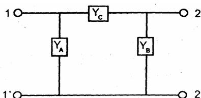
For the two-port network as shown above,  $Y_{12}$  is equal to
