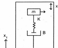
A seismic transducer using a spring-mass-damper system as shown above will have an output displacement of zero when the input  $x_i$  is a
