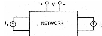
The linear network as shown above has only resistors. If  $I_1 = 8$  A and  $I_2 = 12$  A;  $V$  is found to be  $80$  V.  $V = 0$  when  $I_1 = -8$  A and  $I_2 = 4$  A. Then the value of  $V$  when  $I_1 = I_2 = 10$  A, is
