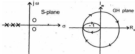
The pole-zero map and the Nyquist plot of the loop transfer function  $GH(s)$  of a feedback system are shown above. For this
