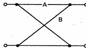
The lattice circuit has the following impedances  $Z_A = 3 + j4$ ,  $Z_B = 3 - j4$ . Then the Z-parameters would be
