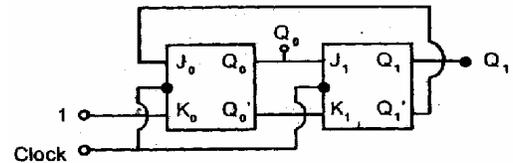
In the circuit as shown above, assuming initially  $Q_0 = Q_1 = 0$ . Then the states of  $Q_0$  and  $Q_1$  immediately after the 33rd pulse are
