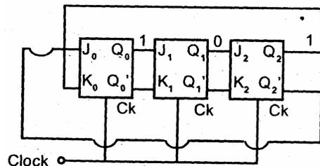
The three-stage Johnson Ring Counter as shown above is clocked at a constant frequency of  $f_c$  from the starting state of  $Q_0 Q_1 Q_2 = 101$ . The frequency of outputs  $Q_0 Q_1 Q_2$  will be
