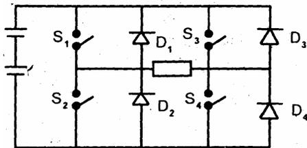
For a single-phase, full-bridge inverter supplying power to a highly inductive load as shown above, the correct sequence of operation of switches and diodes is
