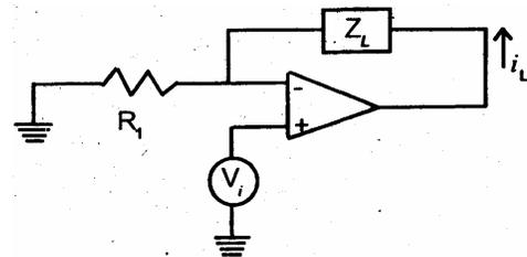
In the op-amp circuit as shown above, the current  $i_L$  is
