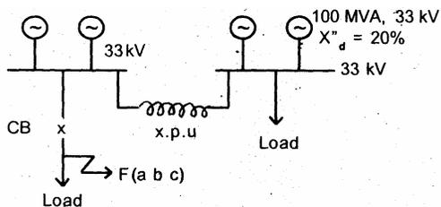
Four identical 100 MVA, 33 kV generators are operating in parallel, as shown above, in two bus-bar sections, interconnected through a current limiting reactor of x p.u. reactance on the
