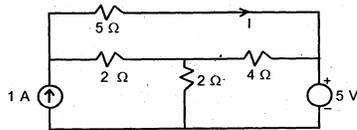
What is the value of current  $I$  in the  $5\Omega$  resistor in the above circuit?
