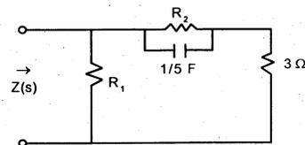
In the above circuit  $Z(s) = 2$  as  $s \rightarrow \infty$  and  $Z(s) = 3$  as  $s \rightarrow 0$ . What are, respectively the values of  $R_1$  and  $R_2$ ?
