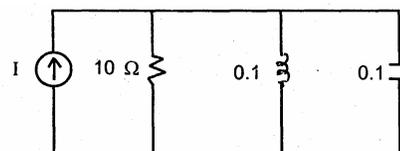
For the above circuit, the current source is sinusoidal with frequency equal to the resonant frequency of the circuit. What is the value of current through the resistor?
