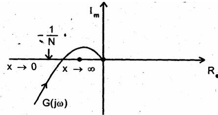
$N$  is describing function of the non-linear device and  $G(s)$  is the transfer function of the linear plant. Which one of the following statements is correct? The limit cycle is
