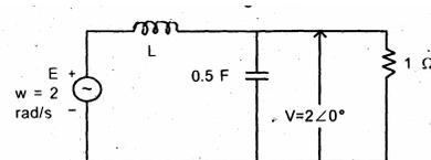
For the circuit shown above, by how much the voltage across the inductor leads the voltage across the capacitor?
