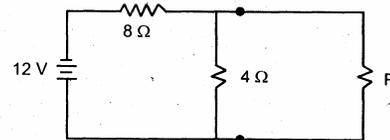
What should be the value of resistance  $R$ , in the above circuit if it has to absorb the maximum power from the source?
