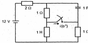
The circuit shown above is in steady state before closing the switch. What is the current  $i(0^+)$  through the switch if the circuit is closed at  $t = 0$ ?
