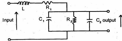
What is the minimum number of states of the network given above in order to determine the complete output of the network over all future time for a given input?
