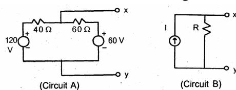
For what values respectively of  $I$  and  $R$ , the circuit B is equivalent to circuit A?
