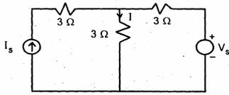
In the above circuit, when  $V_s = 3V$ ,  $I = 4A$ , what is the value of  $I$  when  $V_s = 12V$ ?
