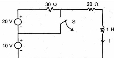
The circuit shown above attains a steady state with the switch  $S$  closed. What is the value of  $I(t)$  for  $t \geq 0$ , if the switch  $S$  is opened at  $t = 0$ ?
