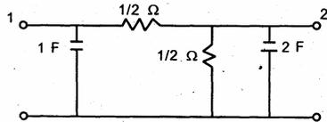
What is the short-circuit natural frequency at port 1 of the above circuit?
