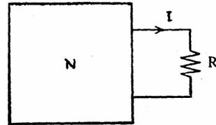
The black-box,  $N$  contains resistors and independent sources. If  $I = 3\text{ A}$  and  $1.5\text{ A}$  for  $R = 0$  and  $2\Omega$ , respectively, then what is the value of  $I$  for  $R = 1\Omega$ ?
