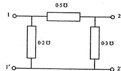
Which one of the following gives the correct short circuit parameter matrix V for the network shown above?
