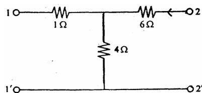
For the 2-port network shown in the figure given above, what is the value of the parameter  $h_{21}$ ?
