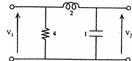
For the two port network shown above, what is the voltage transfer function  $V_2(s) / V_1(s)$ ?
