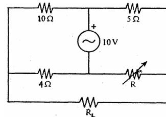
For the circuit shown above, the value of  $R$  is adjusted, so as to make the current in  $R_L$  equal to zero. What is the
