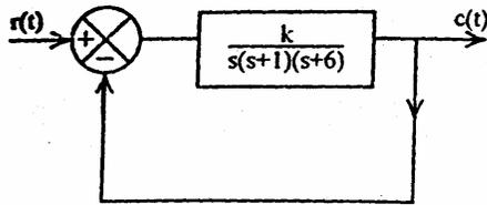
For which of the following values of  $k$ , the feedback system shown in the above figure is stable?
