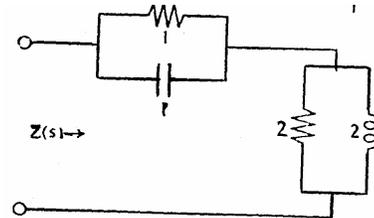
For the circuit shown above, the poles of the driving-point impedance function are at which one of the following locations?
