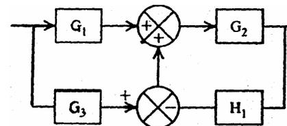
What is the overall transfer function of the block diagram given above?
