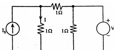
In the circuit given above,  $I = 1\text{ A}$  for  $I_s = 0$ . What is the value of  $I$  for  $I_s = 2$ ?
