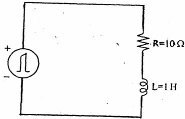
A unit impulse voltage is applied at  $t = 0$  to the R-L circuit shown above while  $i(0^-) = 1$  A. What is the expression for  $i(t)$ ?
