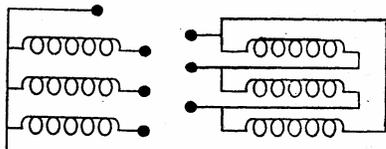
What is the phase displacement between primary and secondary voltages for a star-delta, 3-phase transformer connection shown above?
