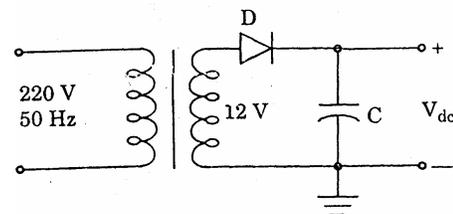
In the rectifier circuit shown above, what should be minimum peak-inverse-voltage (PIV) rating of the diode?
