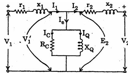
The exact equivalent circuit of a two-winding transformer is given in the figure given above. For affecting simplification, the parallel magnetising branch, consisting of  $R_C$  and  $X_Q$  is shifted to the left of the primary leakage impedance ( $r_1 + jx_1$ ). This simplification introduces the inaccuracy, in the neglect of:
