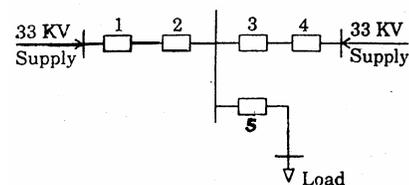
The distribution system shown in figure given above is to be protected by over current system of protection.
