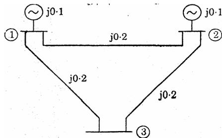
A sample power system network is shown in the figure given above. The reactances marked are in pu. What is the pu value of  $Y_{22}$  of the Bus Admittance Matrix ( $Y_{BUS}$ )?
