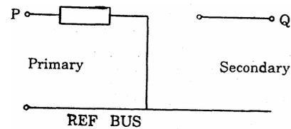
A zero-sequence network of a 3-phase transformer is given above.  $Z_0$  is the zero-sequence impedance of the transformer. What is the type of transformer connections?
