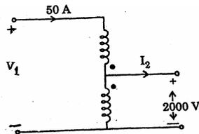
A single-phase, 10 kVA, 2000/200 V, 50 Hz transformer is connected to form an auto transformer as shown in the figure given above. What are the values of  $V_1$  and  $I_2$  respectively?
