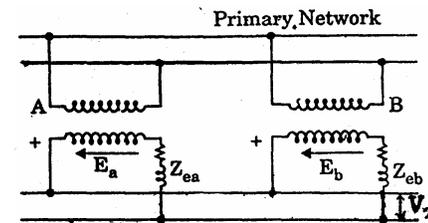
Two single phase transformers A and B are connected in parallel, observing all requirements of a parallel operation, except that the induced voltage  $E_a$  is slightly greater than  $E_b$ ;  $Z_{ea}$  and  $Z_{eb}$  being the equivalent impedances of A and B, both referred to the secondary side.
