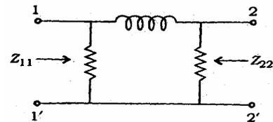
If the driving-point impedance  $Z_{11}$  of the network shown in the figure above is given by  $Z_{11} = k_1 \left( \frac{s+3}{s+8} \right)$  then what is the driving-point impedance  $Z_{22}$  ?
