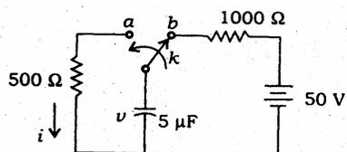
At  $t = 0$ , the switch  $k$  is thrown from  $b$  to  $a$  of the circuit as shown above. What are the values of  $v(0^+)$  and  $i(0^+)$ ?
