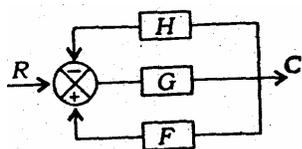
For the feedback system shown in the figure above, which one of the following expresses the input-output relation  $C/R$  of the overall system
