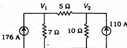
In the circuit shown above, what is the voltage across  $5 \Omega$  resistor ?
