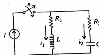
In the circuit shown above, the constant current source of value I is switched on at  $t = 0$ . What are the values of currents  $i_1$  and  $i_2$  at  $t = 0$ , with zero initial conditions ?
