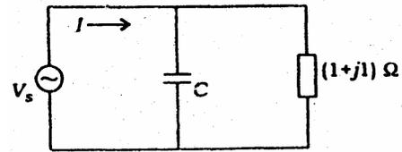
In the circuit shown in the figure above, for what value of C will the current I be in phase with the sinusoidal source voltage  $V_s = \sin 2t$ ?
