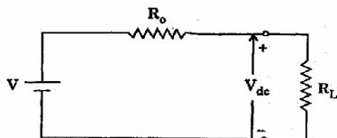
The circuit shown above is the Thevenin's equivalent circuit of a centre-tapped full wave rectifier with diode forward resistance  $R_f = 100 \Omega$ , transformer secondary coil resistance  $R_s = 30\Omega$ , peak input voltage  $V_m = 10 \text{ V}$ .
