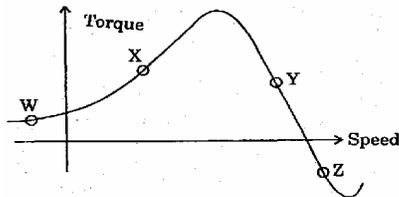
Which of the points on the torque-speed curve of induction motor represent operation at a slip greater than the 1?
