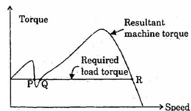
The required load torque line intersects the resultant torque- speed characteristic of a 3-phase squirrel cage induction motor at points P, Q and R as shown in the figure above. Which is/are the stable opening point(s) ?
