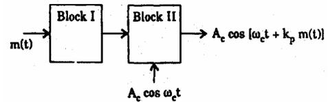
Which one of the following sets correctly describes the Block I and Block II in the diagram given above?
