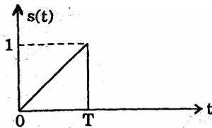
Which one of the following is the impulse response of a matched filter for a signal  $s(t)$  of the type shown above?
