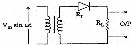
Consider the circuit given above where  $R_f$  is the diode forward resistance and  $R_L$  the load resistance. What is the average rectified current equal to ?
