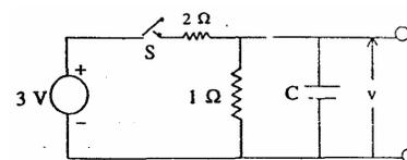
In the network shown above, it is given that  $v = 1 \text{ V}$  and  $\frac{dv}{dt} = -10 \text{ V/s}$  at a time  $t$ , where  $t$  is the time after the switch  $S$  is closed. What is the value of  $C$ ?
