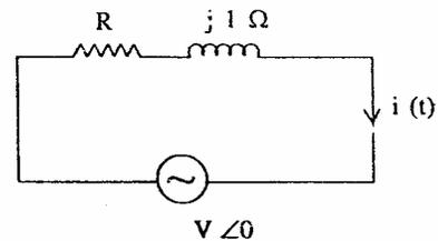
For the network shown above, if the current  $i(t) = \sqrt{2} \sin(\omega t - 30^\circ)$ , then what is the value of  $R$ ?
