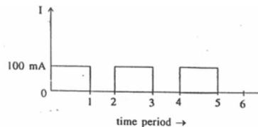
A waveform shown in the figure above, is fed to a d.c. ammeter. What is the reading shown by the meter ?
