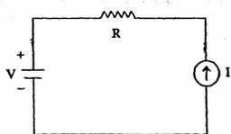
For the network shown in the figure, what is the voltage across the current source I?
