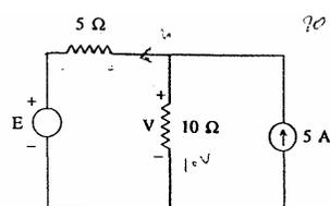
If the voltage V across 10 Ω resistance is 10 V, what is the voltage E of the voltage source in the circuit shown above?
