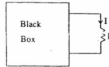
For circuit shown above, the black box contains resistors and independent sources only. The current  $I$  is 3 A and 1.5 A for  $R = 0$  and  $2\Omega$ , respectively. For  $R = 1\Omega$ , what is the current  $I$ ?
