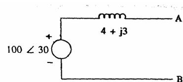
Voltage source is represented as shown in the figure given above.
