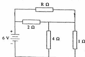
In the circuit shown above, when is the power absorbed by the  $1\Omega$  resistor maximum?
